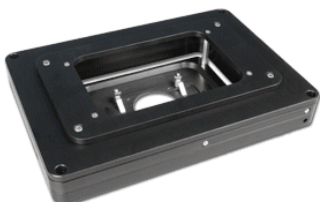
Nano-LPMW with re-entrant slide holder.
