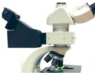
New Prizmatix DMD module (black unit) in-situ
