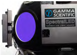
1m integrating sphere fitted with RS-7 illumination
