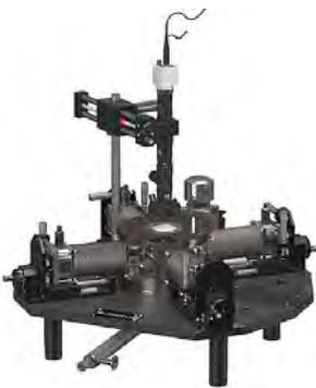
The newly introduced **Lake Shore PS-100** is a pre-configured solution for customers needing a basic, low-cost cryogenic probe station. This packaged system consists of a TTPX probe station set up for four-point triaxial probing, ideal for sensitive, high-impedance DC measurements.
