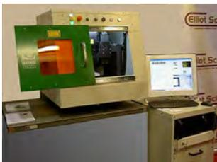
The **Alpha System by Oxford Lasers** is a genuinely capable micromachining system that fits onto a tabletop. The compact Class 1 laser enclosure has a footprint of only 80cm<sup>2</sup>, yet contains many of the features that are usually only available in larger systems. The infrared and visible options facilitate R&D and preproduction machining of metals and ceramics, while an ultra-violet option enables micromachining of some polymers.
