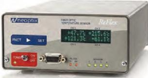
With its 4-channel capability, the fibre optic system based on proven GaAs technology ensures several 'hot spots' can have their temperatures measured simultaneously. This allows for better information on industrial processes or scientific experiments.
