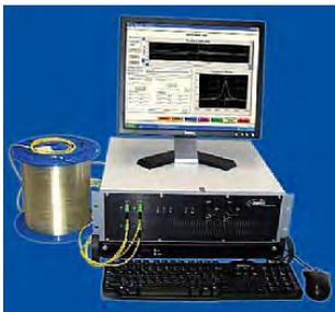
**OZ Optics** has developed **Foresight™**, a sophisticated Distributed Strain and Temperature Sensor (DSTS) based on Brillouin scattering in an optical fibre.
