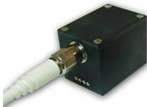
The **MK 25 Monomode Coupler** focusses a free-space laser beam onto an optical fibre by means of a compact piezo-driven aspheric lens equipped assembly. This allows for remote focusing and alignment of systems where traditional hand adjustment would be impractical.
