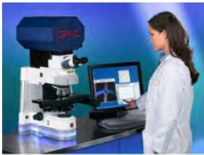
**CRAIC** has developed LambdaFire™, a 64-bit high performance package to control CRAIC microspectrophotometers situated on the manufacturing floor and in the R&D laboratory. Written specifically for Windows 8®, the software is designed to collect, analyse, and process both microspectra™ and images from CRAIC microspectrophotometers running the new OS.
