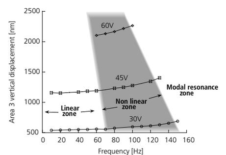
**Figure 3:** The dynamic response of the micro-mirror enables to distinguish the linear, non linear and Modal resonance zone of the micro-system.
