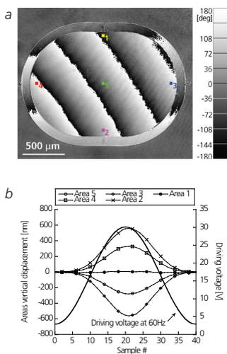
**Figure 1:** (a) Phase image of a 2-axis micro-mirror by Colibrus. (b) Vertical displacement of the areas (left Y-scale) for a sinusoidal driving voltage (right Y-scale) with a peak  $V = 30\text{V}$  at an excitation frequency  $\nu = 60\text{Hz}$ .
