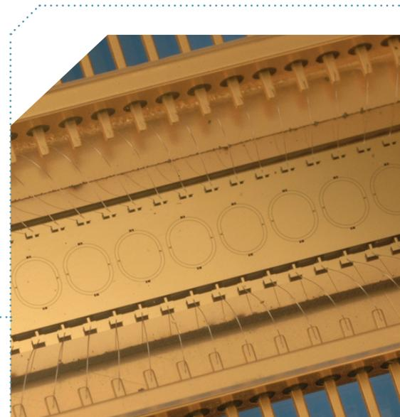
Package mirror array for optical beam steering by Colibrys.
