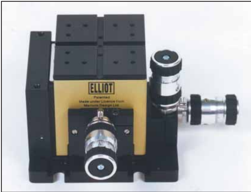
The ELLIOT Gold Series MDE 122 comes fitted with 3 x MDE 216 High Precision Adjusters
