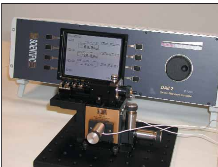
Above: DAI2 with Elliot / Martock MDE 2350 Manipulator - Automatic alignment of polarisation-maintaining fibre and devices.
