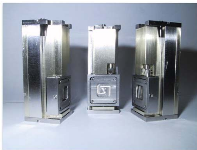
Ultra-compact multi-axis stages can be designed to fit in the most challenging size constraints. This unit is part of an X-ray monochromator and has 2 rotation and 1 linear axes, adjustable from above, in a volume no larger than 20 x 21 x 55mm.
