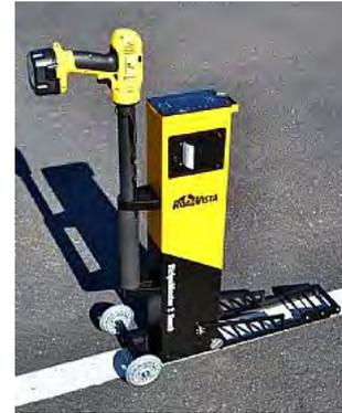
RoadVista's **StripeMaster 2 Touch** is a retroreflectometer designed for use in the field to measure retroreflectivity (RL) of glass beads embedded in white or yellow thermoplastic, traffic paint or temporary marking materials.
