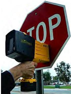
The **RoadVista 922D** handheld retroreflectometer is designed to measure the retroreflection (RA) of road signs and other materials. It features an annular measurement geometry simplifying the measurement process and meets BS EN 12899-1 and DIN 67520 test specifications.
