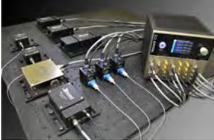
Precise control and stabilisation of a broad range of semiconductor lasers and an associated array of photonics tools is possible via the **Vescent Photonics ICE™** system.
