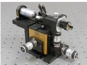
Once again, these positioners come with a choice of adjustment options. Simple thumbwheels, precision micrometers, and piezo driven adjusters are available for use in any combination. An extensive range of add-ons, accessories, and attachments ensure that most applications can be satisfied. If not, [contact us](#) for a custom solution.
