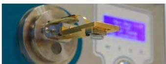
The test sample - maximum size 10 x 10 mm - is affixed to a guitar-shaped carrier with electrical connections made to it from integrated bonding/solder pads. These are routed through the CryoLab for connection to a DAQ interface or CryoLab Breakout Box. A two minute **demo video can be seen here**.
