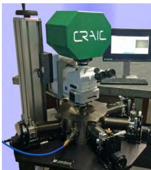
Probe stations are typically used for material studies that include sampling IV and CV curves over a range of temperatures, microwave and electro-optical property responses, magneto-transport characterisation, Hall effect measurements, and so on.
