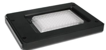
The **Nano-ZL Series** has true flexure guided motion and contains internal position sensing for a resolution of better than 1 nm over the full 500  $\mu\text{m}$  travel range, and sub-nanometer for the shorter 100  $\mu\text{m}$  travel range. In addition to high resolution spatial imaging, the Nano-ZL step response allows entire Z-section acquisitions with minimal photo bleaching. For more information, please **contact us**.
