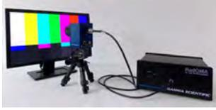
The RadOMA™ range of advanced high-speed spectroradiometers manufactured by **Gamma Scientific**, deliver millisecond measurement speeds, exceptional low-light measurement capabilities, and superior blue-light region sensitivity. The latest versions of the **GS-1290** are now offering wavelength accuracies down to  $\pm 0.2$  nm.
