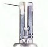
Other key items supplied are: a 635 nm laser excitation source with fibre launch, a 100x 1.25 N.A. oil immersion objective lens, an avalanche photodiode detector, a CMOS alignment camera, and various tuning fork probes (*image above*).
