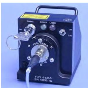
**OZ Optics** has expanded its range of **Visible Fibre Optic Fault Locators** with the addition of a benchtop non-contact tester, the ideal solution for inspecting devices with no connectors on the fibre ends.
