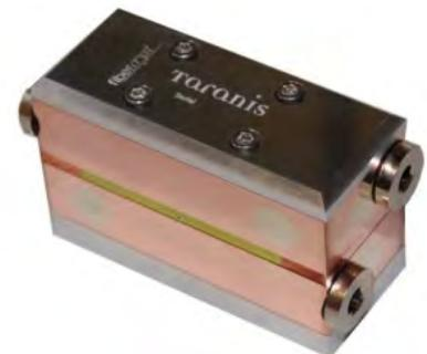
Taranis laser gain modules are water-cooled and can be used with one or two pump diodes, and in single or double-pass geometries. The inherent pump light guiding property of Taranis also makes it ideal for end-pumping configurations.
