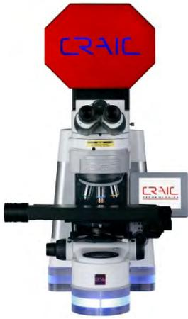
The introduction of new UV laser sources will dramatically enhance the capabilities of the 20/30 PV™ microspectrophotometer from CRAIC Technologies in terms of both fluorescence and photoluminescence microspectroscopy.
