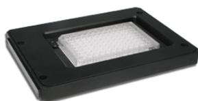
The **Mad City Labs' Nano-ZL Series** are long range, Z-axis nanopositioners specifically designed to hold multiwell plates used in biomedical research. High-throughput single cell fluorescence microscopy and high speed, high resolution confocal imaging can be accomplished while simultaneously adjusting the Z-axis position to remove the effects of multiwell plate irregularities.
