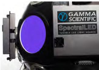
1m integrating sphere fitted with RS-7 illumination
