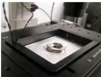
Solid-state heaters can maintain 1 to 50 °C heat above ambient depending on configuration. This allows for a wider range of samples to be studied, and their inherent reliability means less down time during time-lapse experiments.
