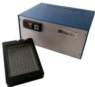
**Intravital Microscopy Imaging System** is specially designed for whole animal viability during extended imaging experiments. There are two independent temperature control channels - one for the removable heated insert, the other for a heated blanket.
