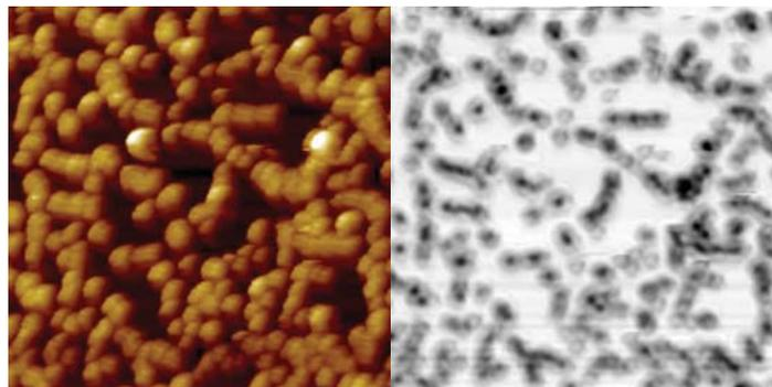
50  $\mu\text{m}$   $\times$  50  $\mu\text{m}$  images of 500nm diameter polystyrene beads on a glass coverslip.
