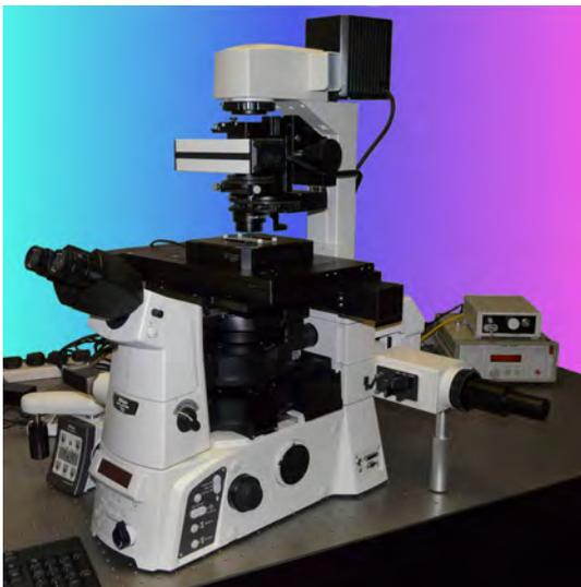
With the Camera Particle Tracking (CPT) option, a high-speed GigE interface camera allows visualisation of the trapped particles through the computer interface. The trap positions are overlaid on the video image to allow easy manipulation of particles.
