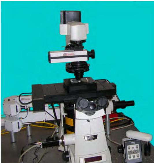
The E3500 system comprises an optical module containing the beam steering optics, external laser source, control module with the drive electronics, microscope interface, PC and unique software. The epifluorescence or camera port of the microscope is used to interface with the optical module and a range of interfaces are available, depending on the make and model of microscope.
