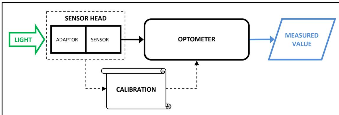
**Figure 1 - Block Diagram, Optometer System:** A Photometer or Radiometer system consists of a calibrated **sensor head** combined with an **optometer**. The sensor head in turn consists of a **basic sensor** combined with an **optical adaptor**. The optometer is programmed with the sensor head **calibration** data, so that the system can display light measurement results in the appropriate units
