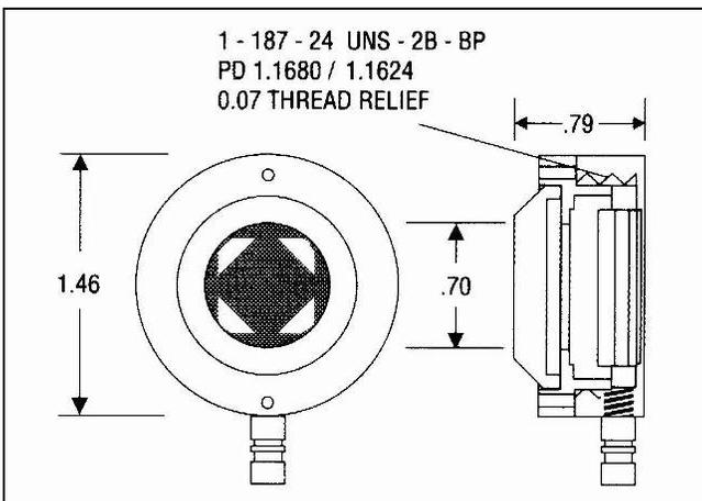
The Model 268P is a low-profile illuminance sensor designed for applications with limited mechanical clearance. Like the Model 211 It consists of a silicon sensor with a spectrally-matched photometric filter and a cosine diffuser to reduce directional sensitivity.
