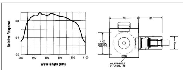
The Model S2575R consists of a Model 262 Flat-response sensor coupled to a Model 2575 Integrating sphere.
