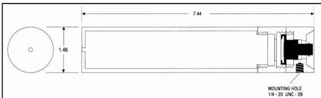
This sensor head makes use of a special fixture to measure lensed LEDs. This attachment fixes the distance and angle between the LED and the detector so that measurement accuracy and repeatability are ensured. *NOTE: For most applications, this sensor head has been replaced by the Model 424 CIE 127 Intensity head. The Model 224 is presently offered to support legacy applications.*
