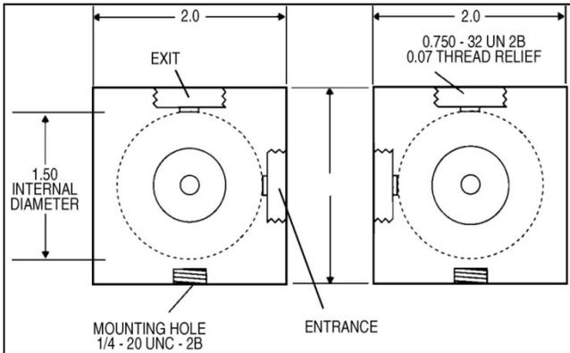
This 50 mm diameter integrating sphere features a 5 mm entrance aperture. This sphere is a favorite for test and measurement of lasers LEDs and fiber-optic illuminators. It is compatible with Miniature Series sensors.
