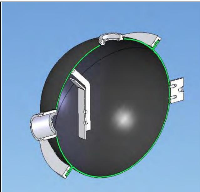
This integrating sphere can be used with Standard Series sensors to determine the luminous or radiant flux of LEDs. The sphere has an internal baffle which makes it ideal for diverging light sources. It includes an input aperture disk with a standard 5mm port and a blank adaptor which can be drilled for other aperture sizes.
