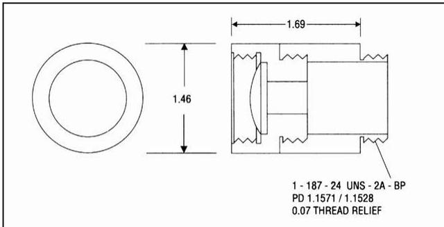
The Model 1153 converts a Model 211 illuminance sensor to a Model 2153 Brightness Sensor. It is intended for users who wish to make both illuminance and luminance measurements with a single sensor.
