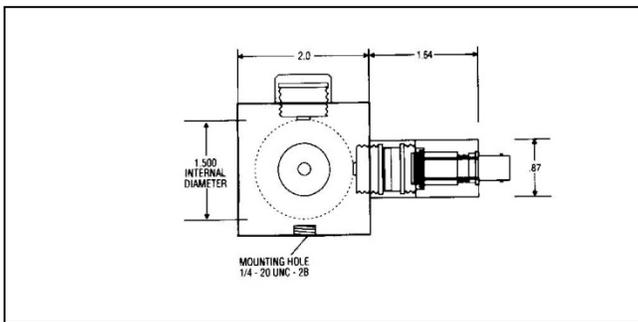
The Model S2575GE consists of a Model 261 Germanium sensor coupled to a Model 2575 Integrating sphere.
