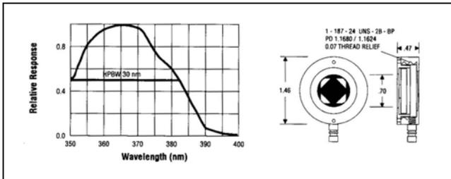
The Model 268UVA is a Low-Profile Series radiometric sensor optimized for measurements in the UVA region (320 - 400 nm).
