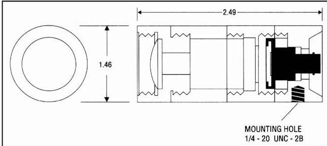
The model 2153 is the UDTi standard luminance head with an integral lens that provides a fixed field-of-view of 13 degrees. It is suitable for measurement of the brightness (luminance) of diffuse surfaces or uniform light sources.
