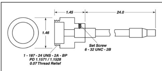
For luminance measurements in difficult to reach places such as in photocopiers or photolithography systems UDT Instruments offers two luminance probes. Both are fiberoptic bundles. The model 116 is two feet long 0.25" fiber core which couple to the Model 211 sensor head.
