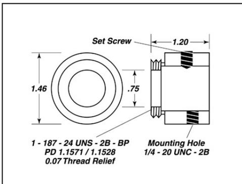
The Model 1718 is designed to couple female-threaded Miniature Series sensors and accessories to male-threaded Standard Series accessories.
