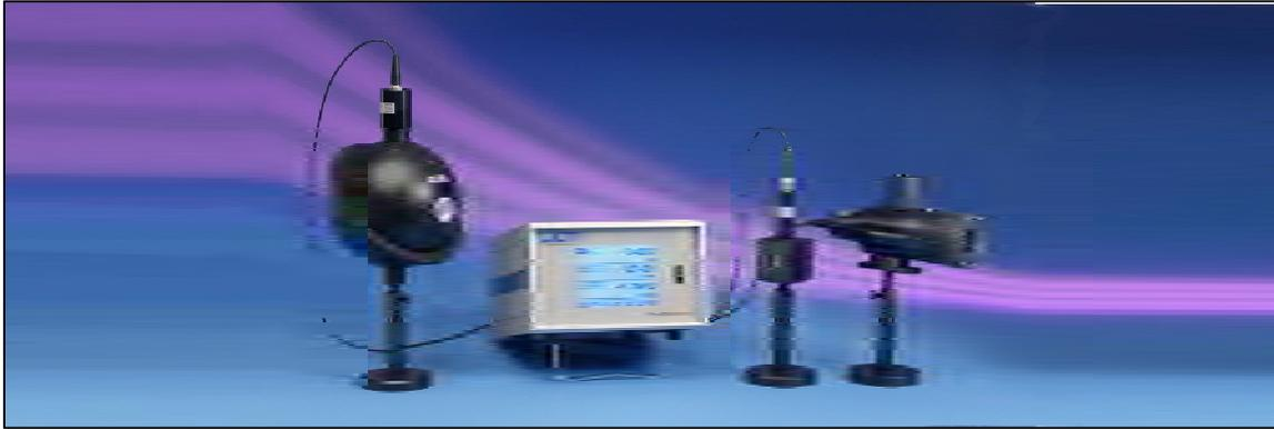
An *optometer* measures the photocurrent produced by a photometric or radiometric sensor, applies a predefined electro-optical calibration factor, and displays the result in optical units. A *photometer* system is built by coupling an optometer to a photometric sensor; a *radiometer* system is built by coupling an optometer to a radiometric sensor.
