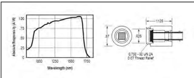
The Model 280 is UDT's Indium-Gallium-Arsenide (InGaAs) sensor. It can be adapted for use with Miniature Series integrating spheres and other accessories.
