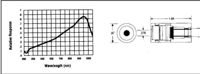
The Model 264 is a Miniature Series sensor specifically designed for laser power measurement. It consists of a Model 260 type sensor with a built-in diffuser and reduced aperture for attenuation of optical power.
