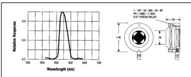
The Model 268BLUE is a Low-Profile Series radiometric sensor optimized for measurements in the blue region centered at 450nm.
