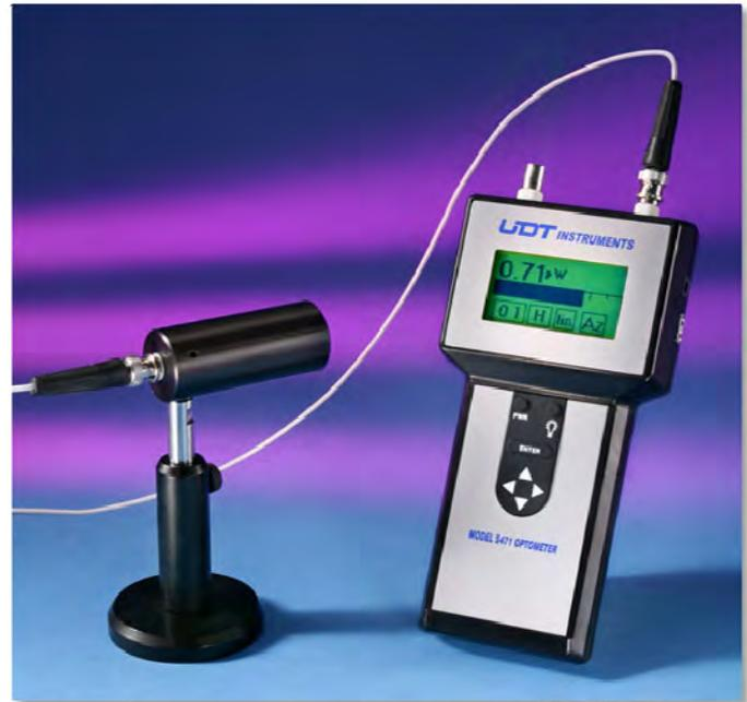
The UDT Model S471 is compatible with the full range of UDTi sensor heads. The unit is shown here configured as a simple spot luminance meter.
