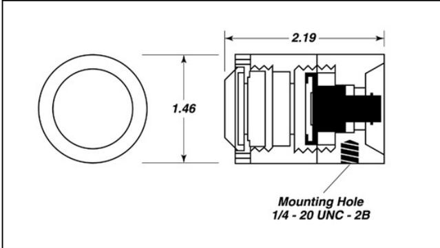
The model 211 is UDTi's universal photometric head as it can be adapted for use with most accessories. It consists of a Standard Series silicon sensor a spectrally-matched photometric filter and a cosine diffuser to reduce directional sensitivity.
