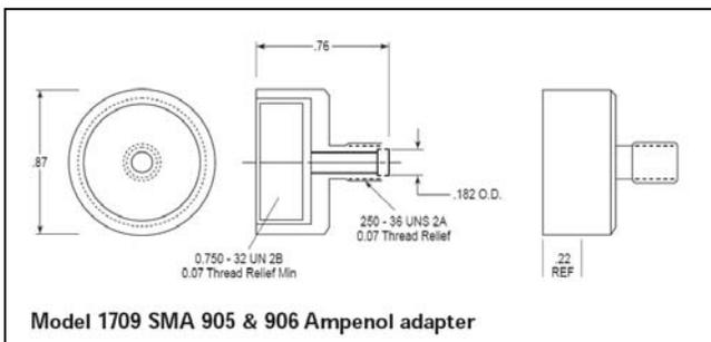
1700-Series Fiber-Optic Adaptors are compatible with UDT Instruments Miniature Series Sensors (Model 260, 261 and 280). Details are provided in the following brochure:
