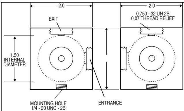
This 50 mm diameter integrating sphere features a 10 mm entrance aperture. This sphere is suitable for testing of larger fiber/bundle diameters. Compatible with Miniature Series sensors.
