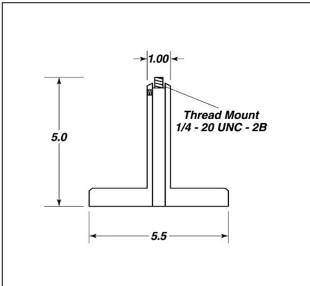
This lab stand has a 1/4-20 threaded post for holding UDTi sensors and accessories. Its extra-heavy base makes it suitable for use with large optical assemblies.
