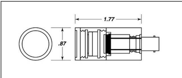
The Model 263 is a scaled-down version of the Model 211 designed for use in confined spaces. It consists of a silicon sensor with a spectrally-matched photometric filter and a cosine diffuser to reduce directional sensitivity.
