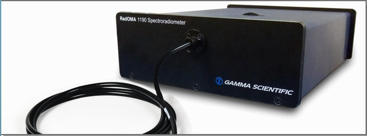
The Gamma Scientific GS-1190 is a high performance, linear CCD array [spectrometer](#), with an 800 kHz readout speed. The spectrometer utilizes a 2048 element detector with 16-bit resolution. Computer interface is USB 2.0. The GS-1190 is ideal for quick and easy [LED measurements](#) for users on a budget. Flexible custom configurations and application support are available for OEM applications.
