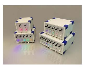
LEDs are ideal for use with various fiber optic spectrometers in continuous, strobe or external triggering measurement mode.
