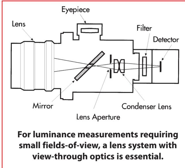
Electronic displays such as CRTs, avionics, and automotive panels are incident directly upon the eye too. But alpha-numeric characters and line detail are generally small. So the measurement system's field-of-view must be limited or focused in order to measure only the lighted portions of the display. This is, by definition, a luminance measurement. So display brightness is usually specified in footlamberts.
