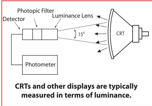
Specifying a **photometer system** is best approached in three steps. First, evaluate the source to determine which measurement technique best applies. Then, select a detector and optical system (**detector head**) that suit the measurement. And finally, match the detector head to the particular electronics which provide the most effective user interface for the application.
