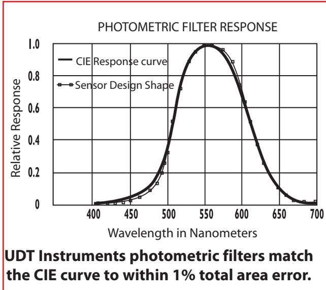
Once the detector's response is fixed, it is calibrated using the transfer of standards technique. This requires a detector of known response, which can be obtained from the National Institute of Science and Technology (NIST). A detector/filter pair is positioned before an optical source with constant wavelength and intensity characteristics (usually a tungsten halogen lamp). The electrical output of the detector under test is then compared to the standard detector's output.
