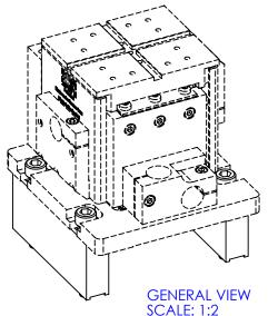
RISER BLOCKS ELEVATE FLEXURE STAGE TOP PLATE FROM A STANDARD OPTICAL AXIS HEIGHT OF 94mm TO 125mm (107 + 18)
