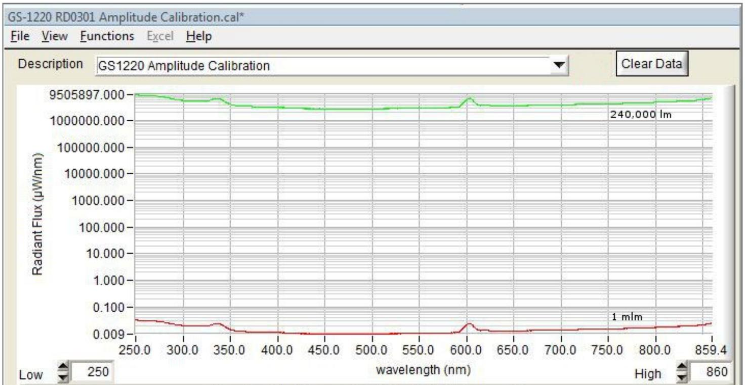
GS-1220 radiant flux-spectral sensitivity range using a GS-IS150 integrating sphere with deuterium and tungsten standards to cover a 250 to 860nm range; 10:1 signal to noise ratio
