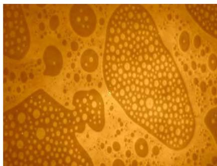
Floating monolayer of Ethylstearate on a water surface with active vibration isolation—image taken with Brewster angle microscope
