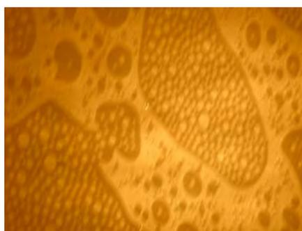
Floating monolayer of Ethylstearate on a water surface without active vibration isolation—image taken with Brewster angle microscope
