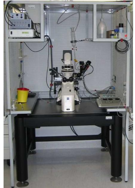
Patch-Clamp set-up on WS\_Vario\_900
