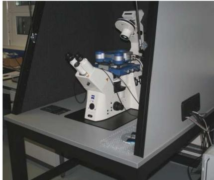
JPK BioScience AFM on WS\_Micro\_1000 with acoustic enclosure
