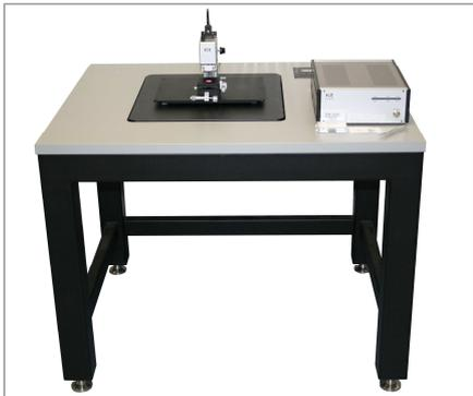
Nanosurf Nanite AFM on WS\_Micro\_780
