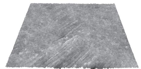
**Figure 2:** 3D representation of the roughness surface of a 1mm diameter micro-ball. The field of view is 100x100 $\mu$ m<sup>2</sup>. Measured values:  $R_a$  = 14.2nm,  $R_t$  = 270nm.
