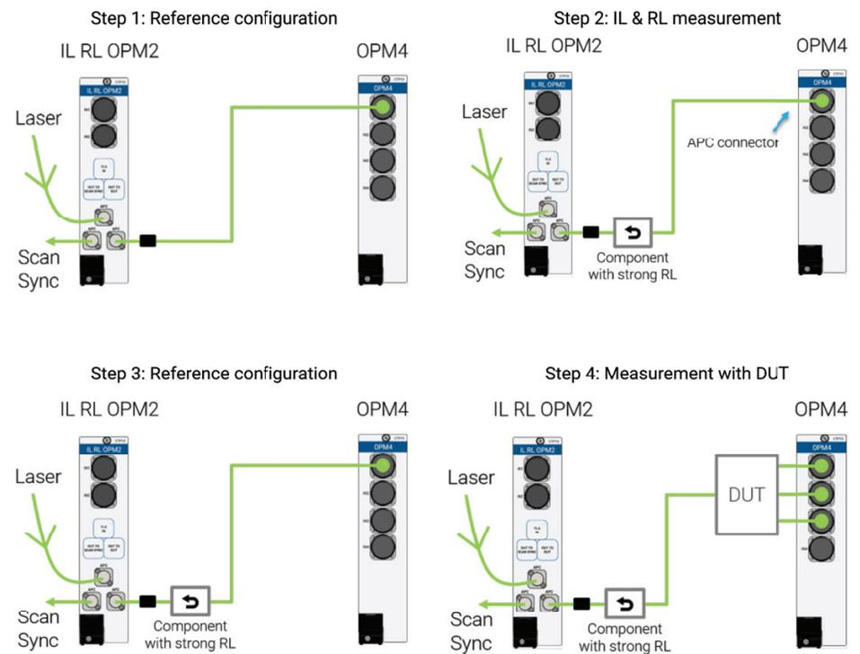
Figure 7. Steps to account for an undesired source of return loss before the DUT.
