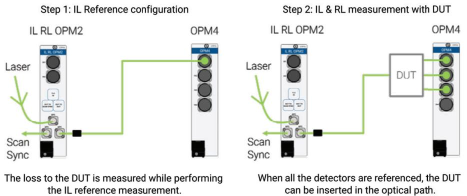
Figure 5. Left: reference configuration. Right: measurement configuration after inserting the DUT.
