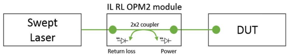
Figure 2. Schematic representation of the return loss measurement principle.
