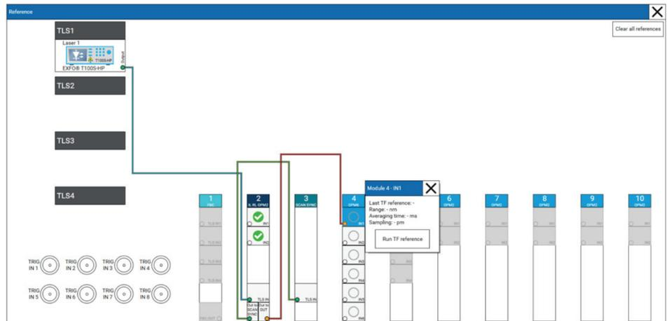
Figure 4. Reference menu of the CTP10 GUI used to reference the system for IL and RL measurements.
