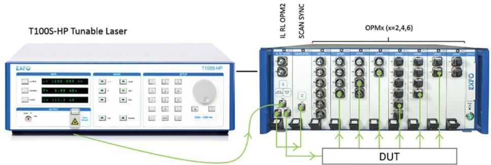
Figure 1. Configuration for swept IL-RL measurement using the CTP10 platform and T100S-HP laser.
