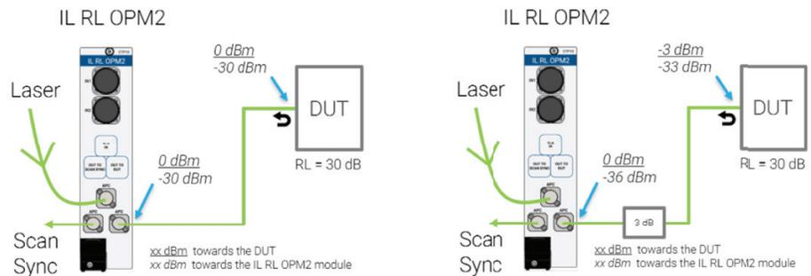
**Figure 3. Left: the 30 dB return loss of the DUT is correctly measured. Right: The 3 dB loss between the IL RL OPM2 module and the DUT will result in a 6 dB error on the measured return loss if not accounted for.**
