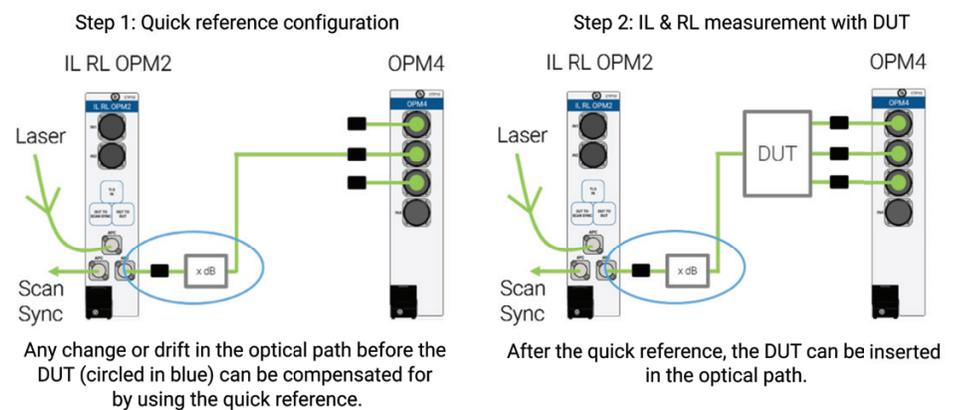
Figure 6. The quick reference can be used to account for changes in the optical path before the DUT.
