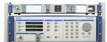
Figure 5. Rack-mountable solution for both (top) CT440 and (bottom) CT440-PDL
