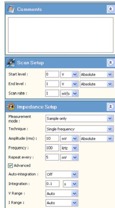
Figure 8 shows a set-up screen for control of the applied waveform. In addition to the control of the voltage, sweep rate and AC stimulus levels, the software also includes a number of other useful features including the ability to control the integration period of the measurement to optimise both speed and accuracy.
