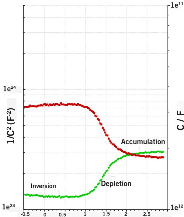
For an n-type device, the capacitance passes through three regions; inversion, depletion and accumulation (green curve Figure 6). In brief,
