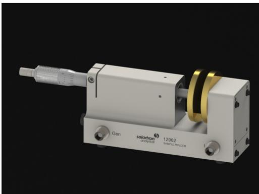
Room Temperature Sample holder for thin film measurements
