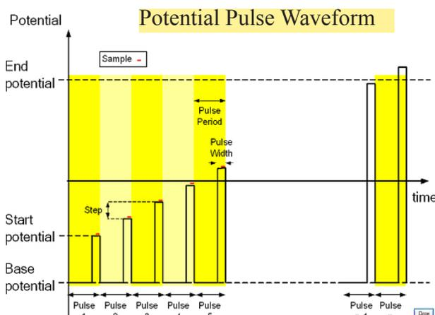
Figure 1 c Description of Potential Pulse Waveform. Normal, Differential and Square Wave options included
