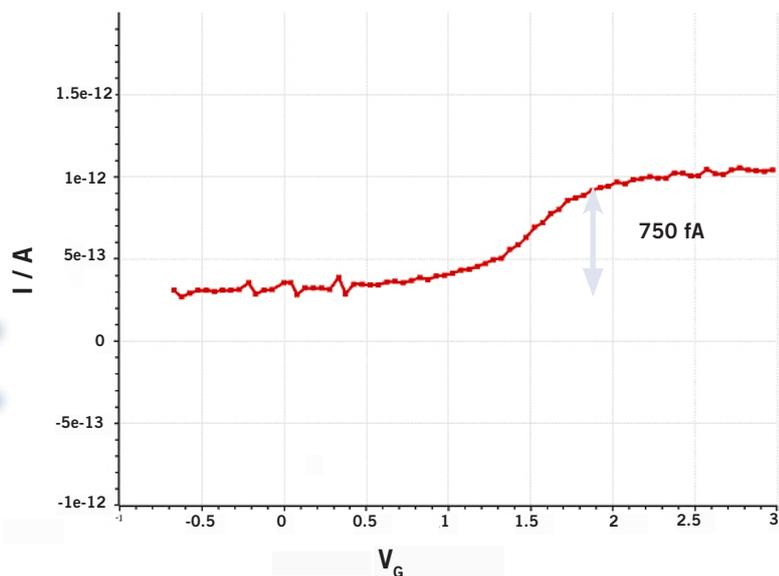
**Figure 3:** I-V curve of a 3N701 MOSFET device (gate to drain/source). This experiment demonstrates excellent stability and resolution of the femto-ammeter module. Note the magnitude of change from inversion to depletion of approximately 750 fA
