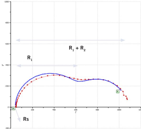
**Figure 12:** Comparison between the theoretical impedance response of the circuit shown in Figure 11 (blue line) vs. the real cell response (red line and dots). There is reasonable agreement between theory and experiment. The impedance values of  $R_1$  (contact) and  $R_2$  (recombination) are shown on the plot. In addition, the series resistance  $R_s$  can be calculated by determining the impedance at the point in which the high frequency measurement intercepts the real ( $Z'$ ) axis.
