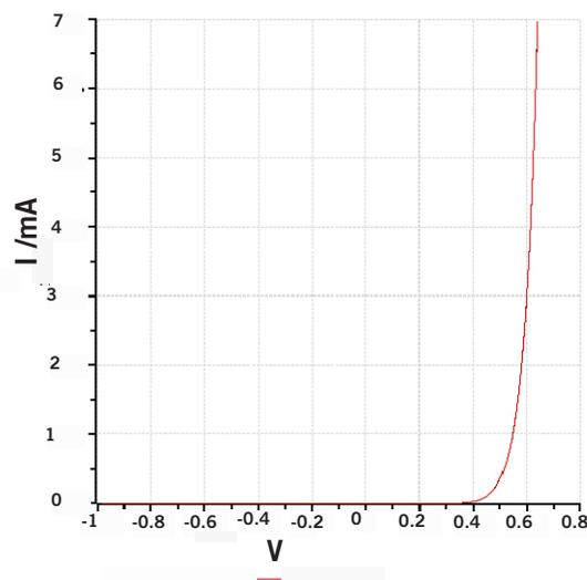
**Figure 4:** I-V curve of a diode operated in forward bias
