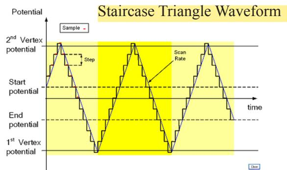
Figures 1 a,b Description of a Triangle Voltage Waveforms (linear and staircase) for I-V characterization.
