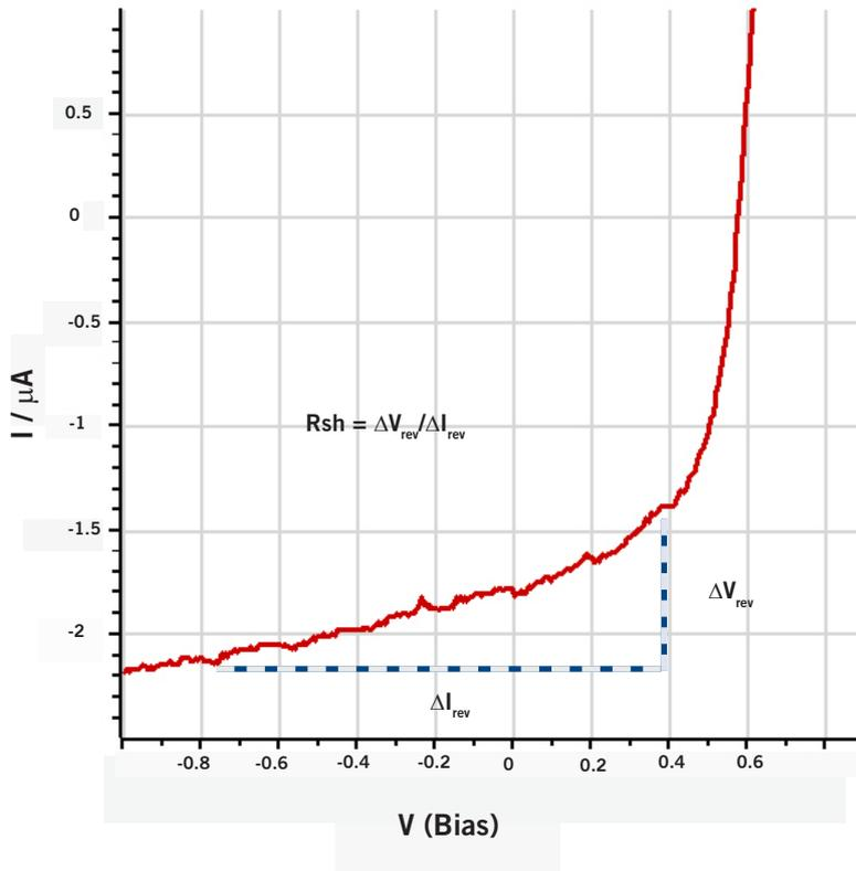
**Figure 5:** Reverse Bias characteristics of an 18 V PV cell indicating method of calculating the shunt resistance. Analysis can be performed in software with regression tool. Note that for very low leakage current devices, Solartron systems have options to increase current resolution down to 0.15 fA.
