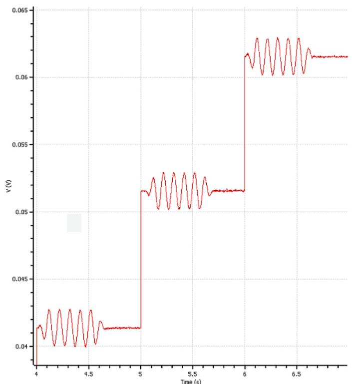
**Figure 7:** AC stimulus level superimposed upon stepped voltage level.
