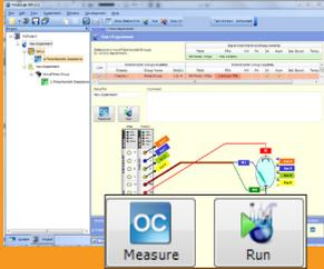
**4** Analyze the data using equivalent circuit fitting, and automatically generate reports using your favorite word processor software
