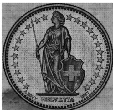
**Figure 2:** Swiss 1/2 Francs coin with inkjet printed insulating spots.
