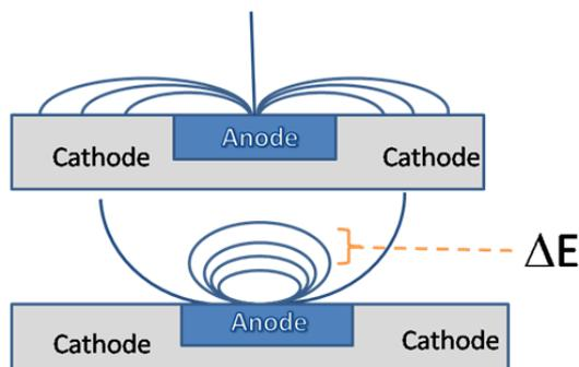
Current path and resulting voltage-fields created from local electrochemical reactions on the surface of a sample.  $\Delta E$  represents the measured value of the SVET experiment.
