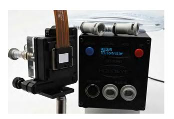
The up-to date display versions of all these SLM platforms use a standardized display packaging with a ceramic stiffener / back plate with excellent thermal conductivity.
