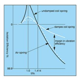
Generally speaking, low amplification at resonance as shown for the plot of a damped coil spring is desirable; however, notice that this is accomplished at the expense of isolation efficiency. Pneumatic isolators with an air spring and damping chamber on the other hand, combines the desirable characteristics of low magnification at resonance and high isolation efficiency as shown the graph.
