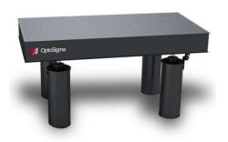
**OptoSigma** OSDVIO optical tables are designed to provide a stable, vibration-isolated platform for precision optical experiments and instrumentation. Constructed with a steel honeycomb core bonded to a ferromagnetic stainless steel top plate, these tables offer high rigidity and flatness, minimizing surface deflection and ensuring accurate optical alignment.
