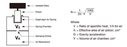
As seen from equation, the natural frequency of the pneumatic isolator depends on the ratio of the piston area to the volume of the air isolator
