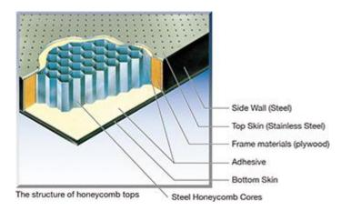
Since all mounting holes on top plates are lead-screw tapped instead of using inserts, deformation or looseness of holes does not occur. The M6(1/4-20) tapped holes are for mounting optical components, arranged in a regular interval 25mm (1").
