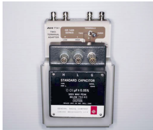
AH TTA1 with GR1409 capacitor installed
