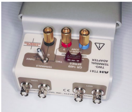
AH TTA1 with a leaded capacitor installed
