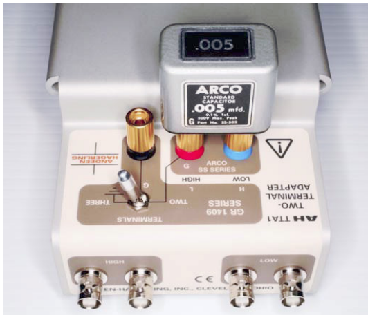
AH TTA1 with Arco capacitor installed
