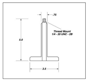
This lab stand has a 1/4-20 threaded post for holding Standard Series sensors.
