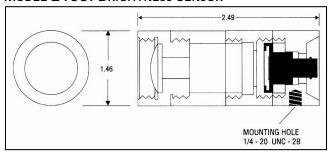
The model 2153 is the UDTi standard luminance head with an integral lens that provides a fixed field-of-view of 13 degrees. It is suitable for measurement of the brightness (luminance) of diffuse surfaces or uniform light sources.
