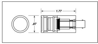
The Model 263 is a scaled-down version of the Model 211 designed for use in confined spaces. It consists of a silicon sensor with a spectrally-matched photometric filter and a cosine diffuser to reduce directional sensitivity.
