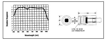
The Model 247 is UDTi's Miniature Series flat response radiometric sensor. It can be adapted for use with Miniature Series accessories.
