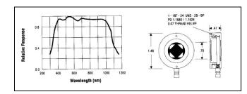
The Model 268R is a Low-Profile Series flat response radiometric sensor.
