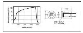
The Model 280 is UDTi's Indium-Gallium-Arsenide (InGaAs) sensor. It can be adapted for use with Miniature Series integrating spheres and other accessories.
