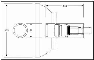
This luminance head was specifically designed for measuring display brightness. Its integral lens provides a fixed field-of-view of 13 degrees and a soft rubber light shade eliminates errors due to ambient light and keeps the display from being scratched during measurement.
