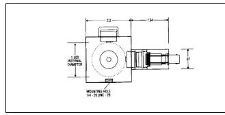
The Model S2575GE consists of a Model 261 Germanium sensor coupled to a Model 2575 Integrating sphere.
