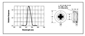
The Model 268BLUE is a Low-Profile Series radiometric sensor optimized for measurements in the blue region centered at 450nm.
