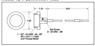
For luminance measurements in difficult to reach places such as in photocopiers or photolithography systems UDT Instruments offers two luminance probes. Both are fiberoptic bundles. The model 124 is two feet long 0.0625" fiber core which couple to the Model 211 sensor head.
