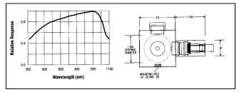
The Model S2575 consists of a Model 260 Silicon sensor coupled to a Model 2575 Integrating sphere.
