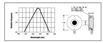
The Model 268UVC is a Low-Profile Series radiometric sensor optimized for measurements in the UVC region (200 - 280 nm).
