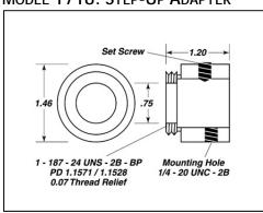
The Model 1718 is designed to couple female-threaded Miniature Series sensors and accessories to male-threaded Standard Series accessories.
