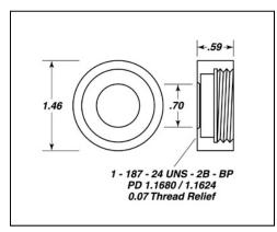
The model 102 Filter Holder holds any 25 mm diameter filter. It is female-threaded on one side for connection to Standard Series sensors.
