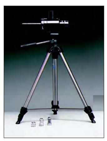
Designed for use in display-measurement microphotometry and telephotometry applications the Model 1706 provides tip tilt and pan capabilities for accurate pointing and alignment. It attaches to any sensor head with a 1/4-20 thread mount and is especially suitable for use with the Model 1120.
