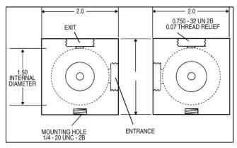
This 50 mm diameter integrating sphere features a 10 mm entrance aperture. This sphere is suitable for testing of larger fiber/beam diameters. Compatible with Miniature Series sensors.
