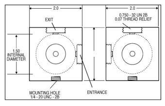
This 50 mm diameter integrating sphere features a 5 mm entrance aperture. This sphere is a favorite for test and measurement of lasers LEDs and fiber-optic illuminators. It is compatible with Miniature Series sensors.
