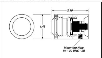
The model 211 is UDTi's universal photometric head as it can be adapted for use with most accessories. It consists of a Series silicon sensor a spectrally-matched photometric filter and a cosine diffuser to reduce directional sensitivity.
