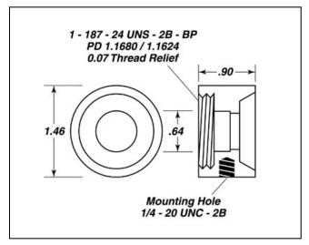
This Universal Sensor Housing holds a standard 1 cm<sup>2</sup> BNC detector package and is a component of UDTi Standard Series sensors. Includes a male-threaded adaptor (Model 108) which connects directly to Standard Series filter holder (Model 104) attenuators and integrating spheres.
