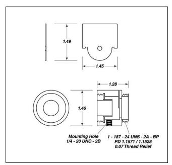
This accessory holds our standard 1cm<sup>2</sup> silicon photosensors. It is provided with five interchangeable apertures.
