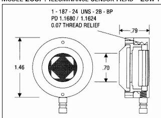
The Model 268P is a low-profile illuminance sensor designed for applications with limited mechanical clearance. Like the Model 211 It consists of a silicon sensor with a spectrallymatched photometric filter and a cosine diffuser to reduce directional sensitivity.
