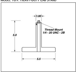
This lab stand has a 1/4-20 threaded post for holding UDTi sensors and accessories. Its extra-heavy base makes it suitable for use with large optical assemblies.
