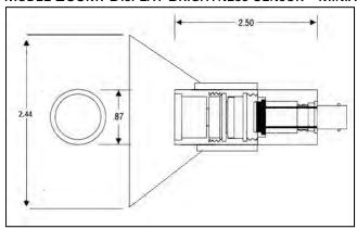
This luminance head was specifically designed for measuring display brightness. Its integral lens provides a fixed field-of-view of 13 degrees and a miniature fixed rubber light shade eliminates errors due to ambient light and keeps the display from being scratched during measurement.
