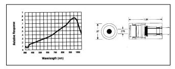
The Model 264 is a Miniature Series sensor specifically designed for laser power measurement. It consists of a Model 260 type sensor with a built-in diffuser and reduced aperture for attenuation of optical power.
