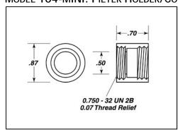
Designed to hold 12.5 mm diameter filters the Model 104-MINI connects male-threaded Miniature Series sensors and accessories.
