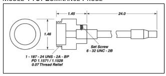
For luminance measurements in difficult to reach places such as in photocopiers or photolithography systems UDT Instruments offers two luminance probes. Both are fiberoptic bundles. The model 116 is two feet long 0.25" fiber core which couple to the Model 211 sensor head.
