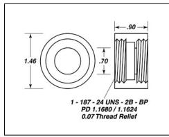
Designed to hold standard 25 mm diameter filters the Model 104 connects male-threaded Standard Series sensors and accessories. While the Model 102 Filter Holder is threaded on one side only both sides of the Model 104 are threaded to permit stacking of accessories.
