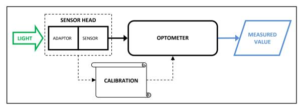
**Figure 1 - Block Diagram, Optometer System:** A Photometer or Radiometer system consists of a calibrated **sensor head** combined with an **optometer**. The sensor head in turn consists of a **basic sensor** combined with an **optical adaptor**. The optometer is programmed with the sensor head **calibration** data, so that the system can display light measurement results in the appropriate units
