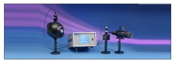
An *optometer* measures the photocurrent produced by a photometric or radiometric sensor, applies a predefined electro-optical calibration factor, and displays the result in optical units. A *photometer* system is built by coupling an optometer to a photometric sensor; a *radiometer* system is built by coupling an optometer to a radiometric sensor.
