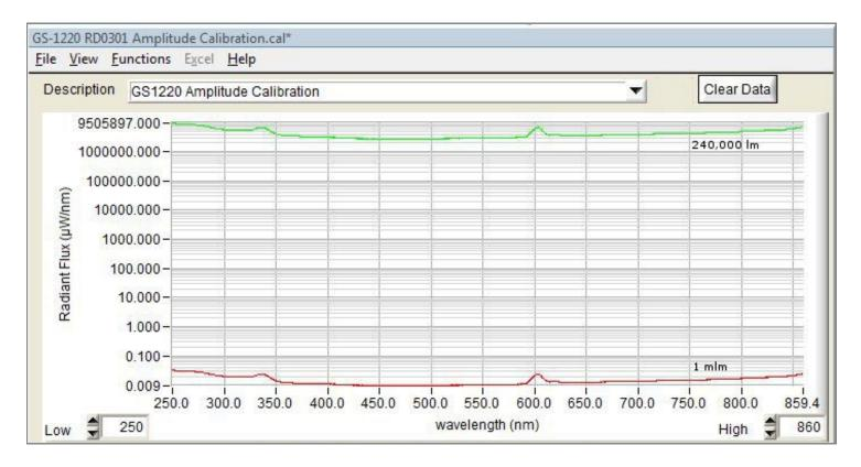
GS-1220 radiant flux-spectral sensitivity range using a GS-IS150 integrating sphere with deuterium and tungsten standards to cover a 250 to 860nm range; 10:1 signal to noise ratio
