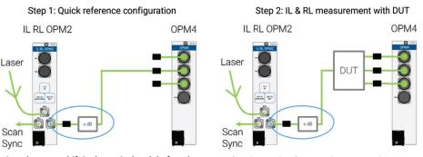
Any change or drift in the optical path before the DUT (circled in blue) can be compensated for by using the quick reference.
