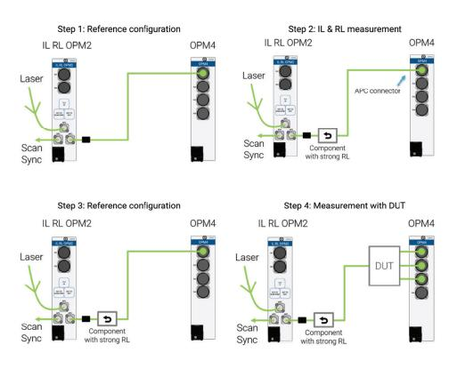
Figure 7. Steps to account for an undesired source of return loss before the DUT.
