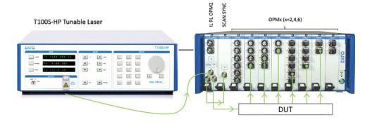
Figure 1. Configuration for swept IL-RL measurement using the CTP10 platform and T100S-HP laser.
