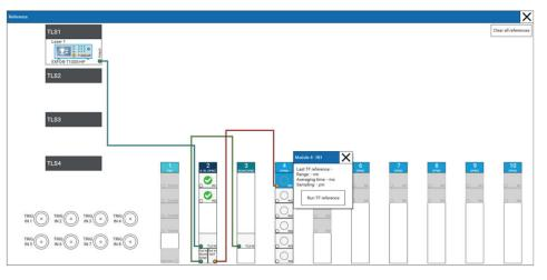
Figure 4. Reference menu of the CTP10 GUI used to reference the system for IL and RL measurements.
