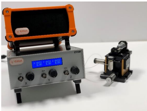
Dali 4- Automated fibre/ device alignment system
