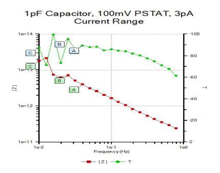
Figure 1. Impedance plot from the 1 pF capacitor in the high impedance test box.
