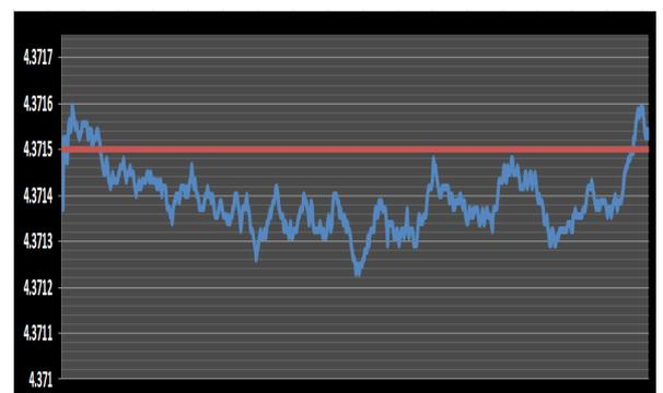
Voltage vs. Time Trace for a requested 4.3715 V ( — )
