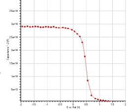
Figure 4. Mott-Schottky plot of solid-state solar cell derived from C-V measurements.
