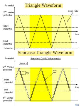
Figure 2a and b Description of a Triangle Voltage Waveforms (linear and staircase) for I-V characterization. Start, 1st vertex, 2nd vertex and end potentials are defined by the end user in the software. Multiple cycles can be used to determine if the system is stable under a varying load. Scan rates from 100  $\mu$ Vs<sup>-1</sup> to 1M Vs<sup>-1</sup> are available with data acquisition up to 1 Million samples per second.
