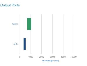
Oria Blue generates two synchronised beams that simultaneously provide the converted output in the near-UV and visible spectrum (340-550 nm) and the unconverted fundamental in the IR spectrum (680-1100 nm). The full spectrum is covered by a single set of optics for maximum flexibility.
