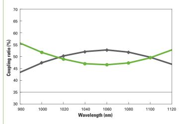
Typical fiber coupler used in OCT systems requires broadband response in the wavelength of interest (courtesy Gooch and Housego).
