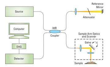
Schematic of a generalized OCT system. One of many modern interferometry based precision sensing systems.
