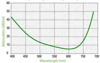
Nufern offers a suite of select cutoff SM and PM fibers that cover the 350 to 850 nm wavelength range ideally suited for spectroscopic applications. Nufern's PM-S405-XP fiber covers the RGB wavelength range offering low attenuation necessary for many medical spectroscopic applications.
